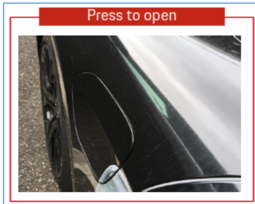
Charger socket access on vehicle
